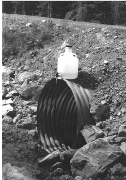
Figure 1. Mariotte bottle injecting into culvert.
