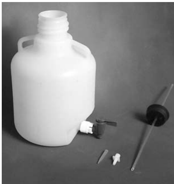
Figure 1. Materials required to construct Mariotte bottle. From left to right: 10-L carboy, pipette tip, Quick Disconnect Connector, rubber stopper with Plexiglas tube inserted.
