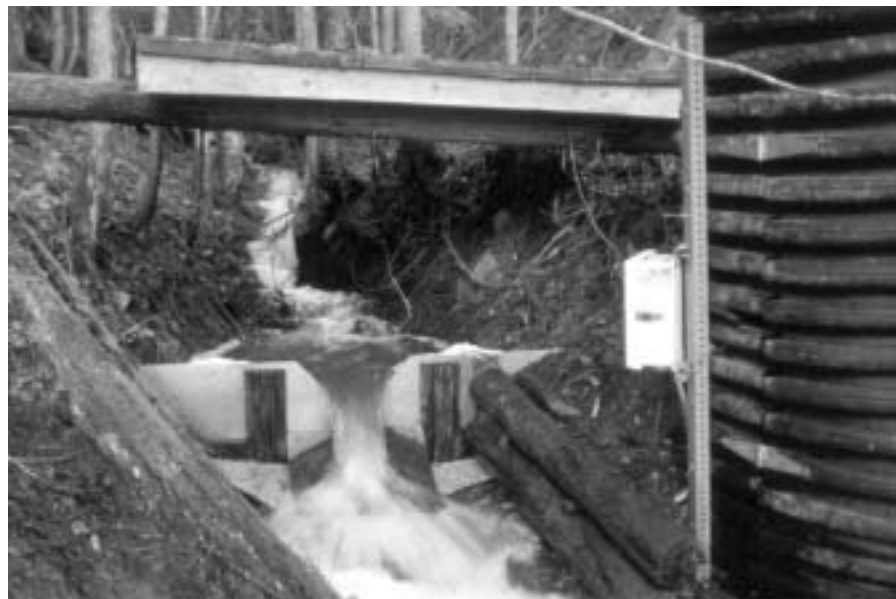
Figure 1. A steep stream unsuitable for gauging with a current meter. Because of the significant approach velocity, a standard weir equation may not be accurate, and the weir should be rated using discharge measurements.
